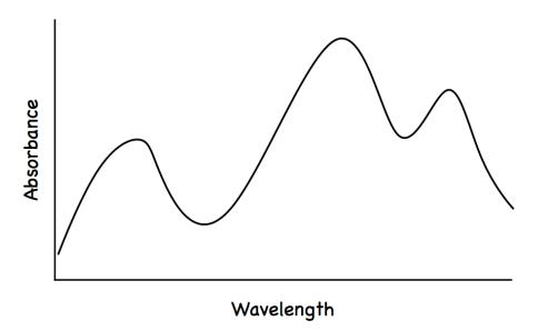
After finding the best wave length we can then proceed to zero the spectrophotometer and measure the absorbance of different concentrations.
