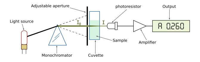
One of the first things we'll need to do to use the spectrophotometer is determine the best wave length to use. To do that we'll need to determine the absorbance of the sample at different wavelengths and graph that.
